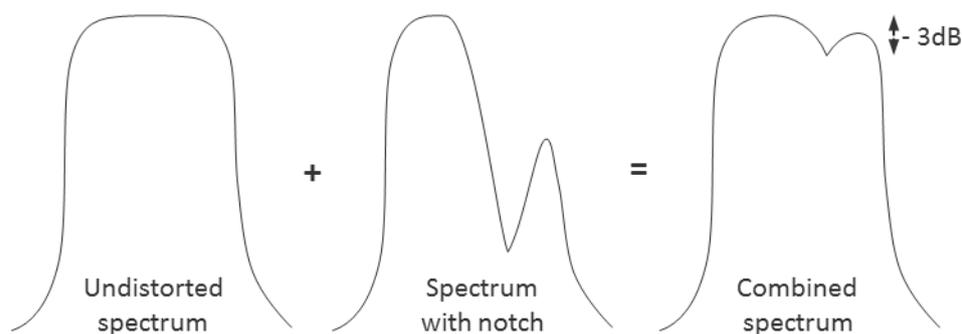
Figure 5 – Combining RF spectrums showing reduced notch of the combined spectrum
