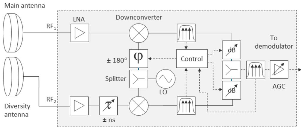
Figure 8 – Principle block diagram of an IF combiner space diversity receiver
