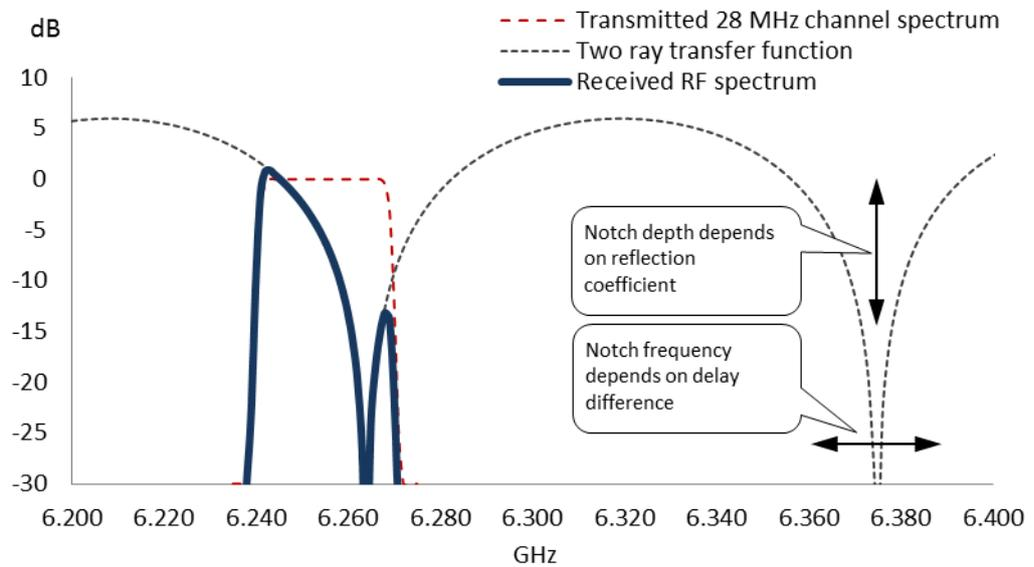
Figure 2 – Distortion of received signal in a two-ray propagation model
