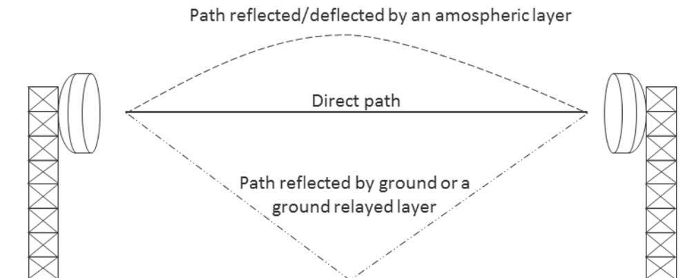
Figure 1 – Principle of multipath propagation
