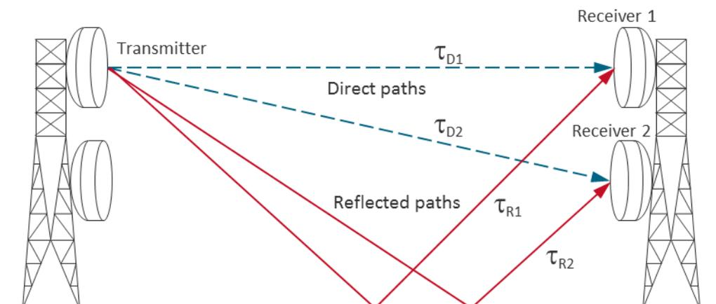
Figure 4 – Multipath space diversity arrangement (one direction shown)
